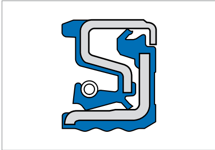
Fig.1 Simmerring Cassette Seal Type 1
