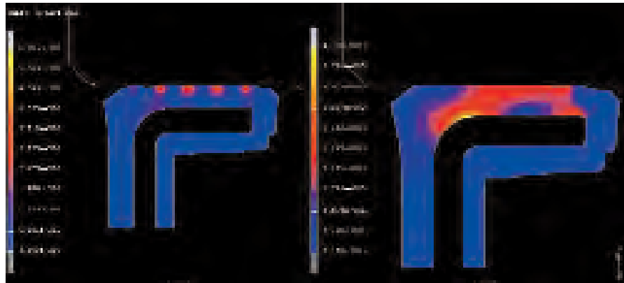
Simulation of static sealing in the housing bore using the finite-element method
